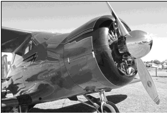
The 450 hp Pratt & Whitney radial engine.
