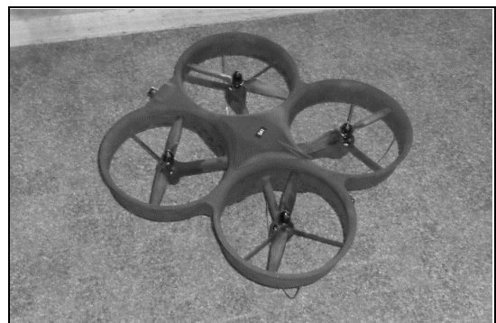
The CyberQuad – with its four ducted props.
