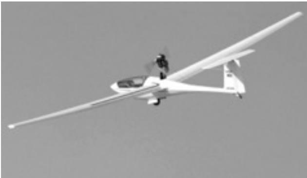
The PIK-20 with the motor extended.
