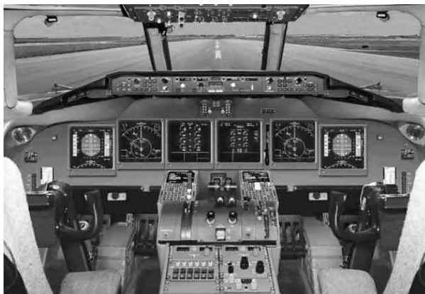
A typical 'glass cockpit' in a modern passenger jet.
