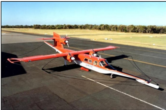
A geophysical aircraft with “stingers” and a diamond aerial.
