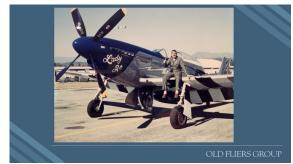
This aircraft will bite if you don't follow its unique procedures. For instance, on take-off, as the tail rises, the gyroscopic effect of the large propeller will swing the nose strongly to port.
